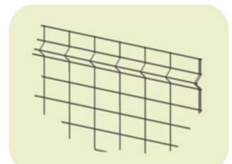
The horizontal 3D profile in the MonkeyMESH™ provides strength and rigidity to the mesh panel.
