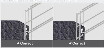
When inserting the Panel into the top Brackets, ensure that one of the three top-most horizontal wires is positioned into the top catchment slot of the Brackets.
